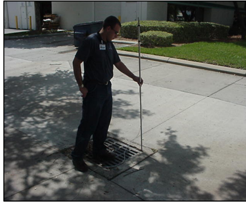
Figure 16: A manhole rim used as an external reference point.
